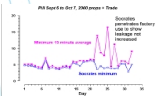
Daily plot of minimum night-flows. Socrates shows true minimum flow and separates out trade flows. High night flow is due to usage and not leakage
