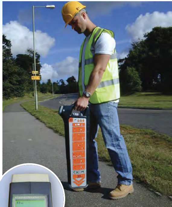
LCD meter displays signal strength, mode, depth and battery condition
